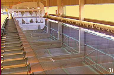
Photo PILKINGTON Freyming-Merlebach Factory 1) Loading of raw materials 2) and on cover: molten glass on the surface of the tin bath 3) Glass ribbon on float bath
