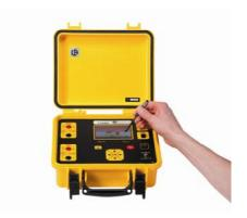
The FTV200 also offers an exceptional ergonomic feature: its integrated library containing the specifications of several thousand different types of solar panels! The tests are validated by comparing the stored curves (STC) with the measurement curves (OPC). The colour screen makes it even simpler to read the result.
