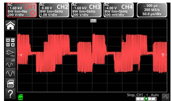
Above: use of envelope selection in OSCILLOSCOPE mode to view the shape of the pulses.
